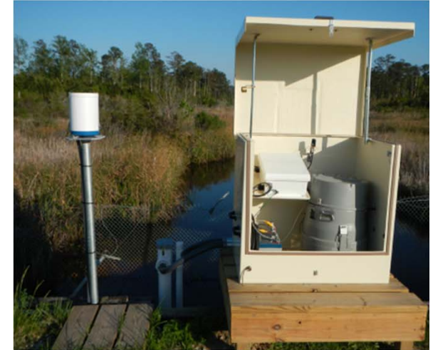
YSI Systems Stormwater monitoring enclosure with solar power, automated water sampler, cellular based real-time data/event notification, WaterLog rain gauge, EXO2 water quality instrument and a SonTek IQ flow sensor.
