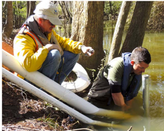
YSI field technicians installing protective casings for a EXO water quality sonde and discrete water sampler suction line.
