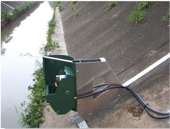
SonTek IQ acoustic Doppler profiler based open channel/ non-full pipe flowmeter being installed in a typical stormwater culvert.
