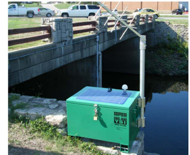
Portable water quality stormwater site in Kansas equipped with WaterLog GOES satellite data delivery, EXO2 water quality instrument and solar power.
